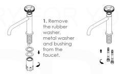
2. Screw and hand tighten the hot and cold flexible hoses to the faucet. So not use a wrench to tighten hose as this may damage the hose and/or the hose threads
