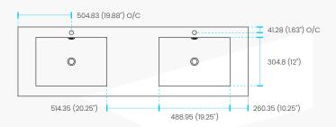
Thickness: 0.38" (9.53) | Faucet Hole ø: 1.38" (35) | Drain Hole ø: 1.75" (44.45)
